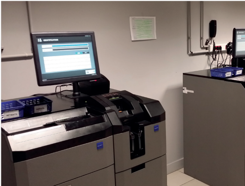
At nine Leclerc hypermarkets, notes are collected in special interface cassettes which automatically feed into cash recyclers at the back office. © Glory
