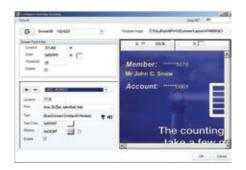
Overlay screens can be added on top of QuickChange's default customer screens to provide additional information to the user during the counting process.
