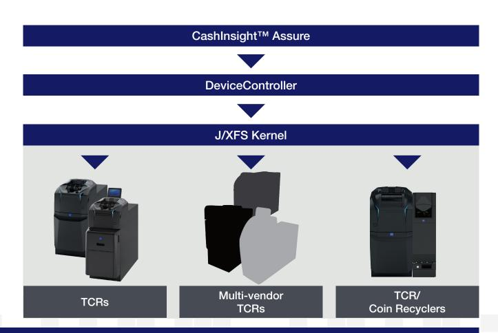
The n-tier architecture of CashInsight Assure brings multi-vendor and multi-device capabilities in a standardised but flexible form, while building on a proven, reliable middleware solution. New devices can be introduced by adding new drivers, without impacting teller workflows. Clear boundaries ensure that each software layer delivers de-coupled capabilities that ease support, maintenance and future development; all designed with today's distributed computing environments in mind.
